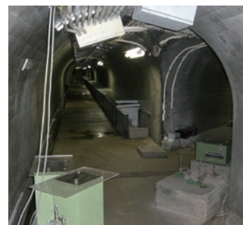
Instruments housed in a tunnel to observe subtle strain of Earth's crust
