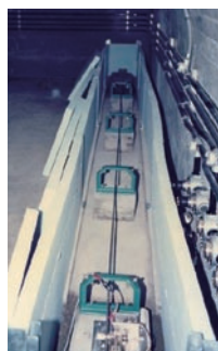
Instruments housed in a tunnel to observe subtle strain of Earth's crust
