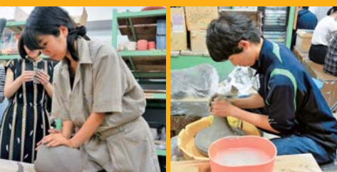
Yuki kneads clay for a pot (left) while Kazutoshi throws a pot on the wheel
